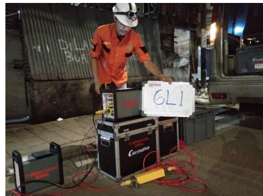
Figure 6. ERT Data Acquisition
